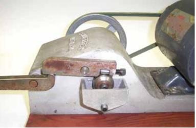
by adding weights to a handle rather than hand pressure.Some bearing machines have a meter to measure current drain on the motor to indicate relative efficiency.
