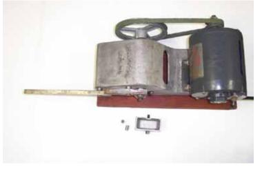
diminishes, rapidly apply load to seize the parts. You have just made the test oil fail, and you can remove the bearing roller and show your audience a big nasty wear scar.
