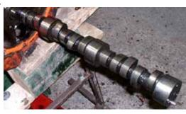
V-8 engines with flat tappets are particularly susceptible to failure, or maybe it just appears that way because there are more of them, but a lot of failures have been reported.<sup>5,6,7</sup> These engines provided long service life with the old oil formulations they were designed for, but failure rates have increased with today's low-phosphorus passenger car motor oils.
