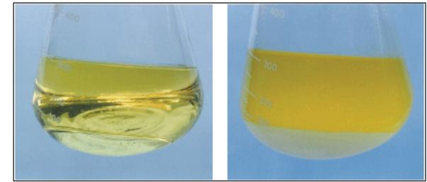
Phase Separation happens when ethanol blended fuels pick-up more water than the ethanol can absorb, reaching its saturation point. At this time (as shown on the right) the ethanol and water will separate, actually coming out of solution and forming two distinct layers in the tank.
